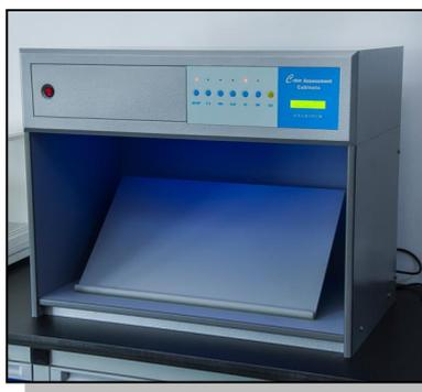
Under ultraviolet light to detect color of the sample.
